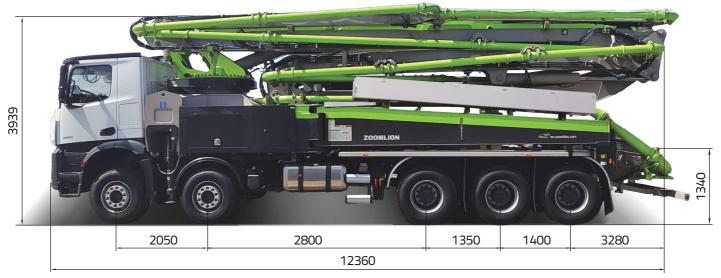
Note: Standard version. Dimensions and weights depend on truck, pump model and equipment. Dimensions in mm. Example based on Mercedes-Benz Arocs 5 4751. For illustration only. Actual products may vary.
